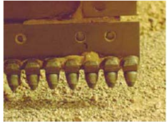
Figure 22. Individual carbide steel cutting bits
