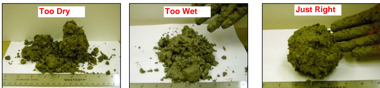
Figure 18. DSA Moisture Field “Test”.
