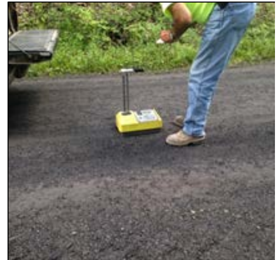
Figure 17. Compaction Testing with Nuclear Density Gauge
