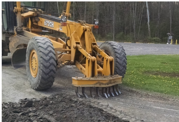
Figure 27. Grader equipped with scarifier teeth.
