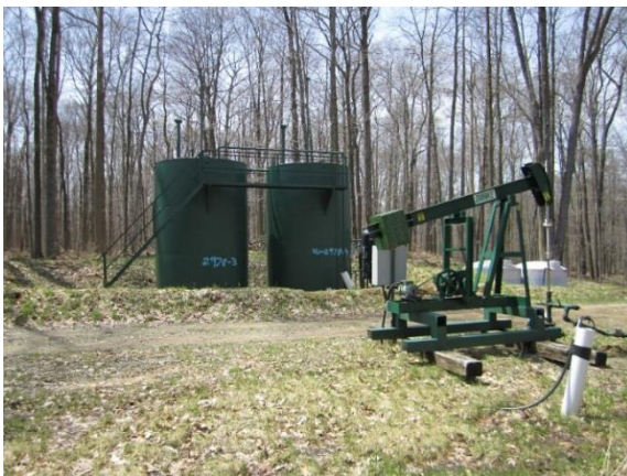
Figure 5 tank battery and pumping station
