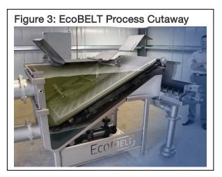
EcoBELT's patent-pending, engineered belt support structure facilitates maximum use of available surface area without losses from media backing and structural support members, while minimizing stresses to the belt media and extending the belt lifecycle.
