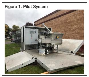
pumps for priming the influent lines to the pilot unit. The pilot system is pictured in Figure 1. The control panel housed all controls for instrumentation and the automated operation of the pilot.
