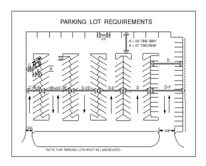
(2) <u>Parking Table.</u> The size and spacing specifications for required offstreet parking facilities shall be taken from the diagram and table below:
