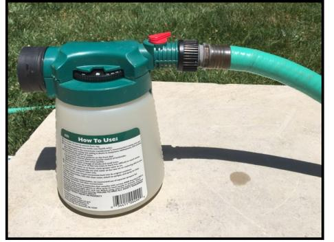
Hose Sprayer—must have a vacuum breaker or an anti-siphon spigot when using this. Otherwise, you run the risk of the chemicals getting into your home, causing a cross connection.
