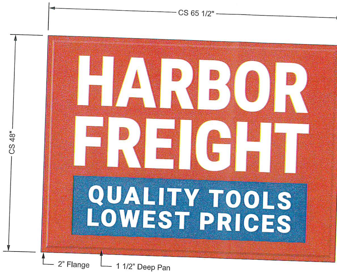
PYLON ELEVATION - Sign Type (B) (QTY:2) Pan-formed face with vinyl graphics. Scale: 1" = 1'
