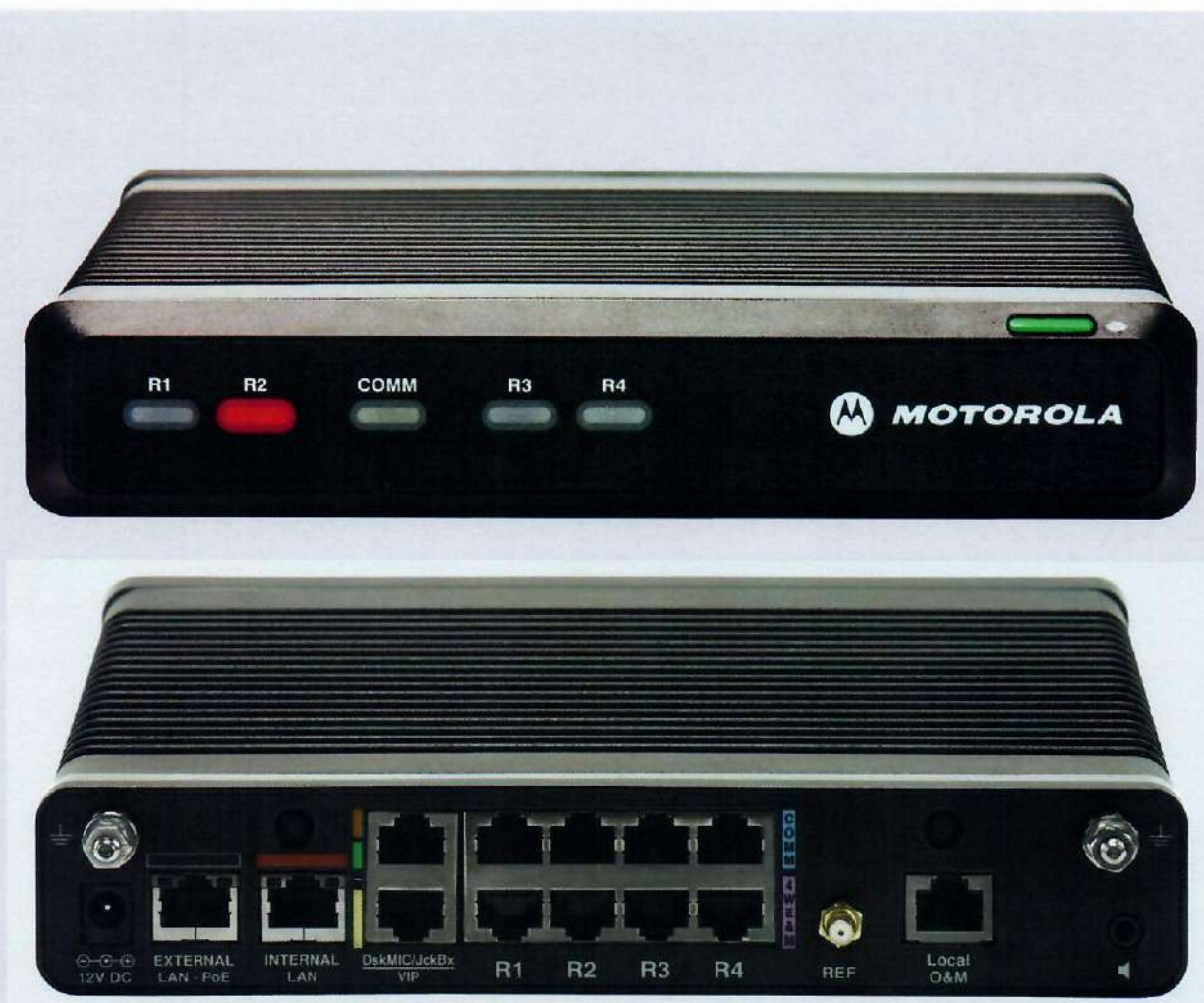
The MCD 5000 RGU connects radios to the MCD 5000 Deskset over your IP network
