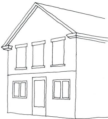
Figure 16 — Converted residential building with windows that are too small, poorly proportioned, and in a modern style that does not fit the design of the building.
