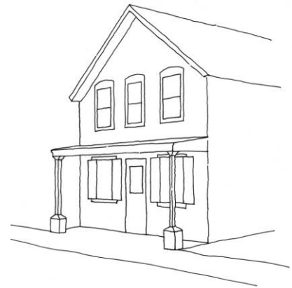
Figure 13 — An original, well-proportioned façade with residential-scale windows, columns, and canopied entrance.
