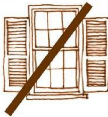
The louvered shutters are the incorrect size for the window Not Recommended
