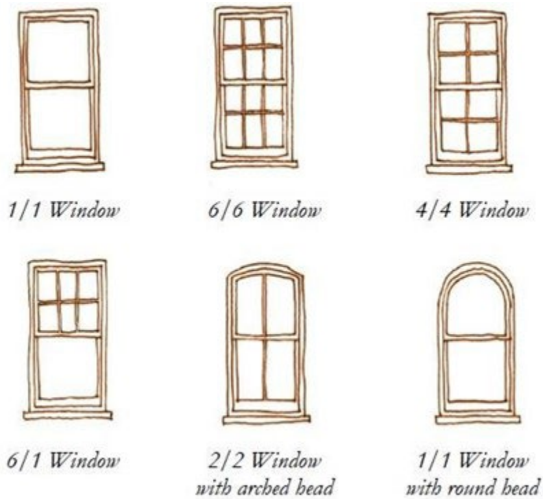
Figure 45. Typical wood window configurations shown above. Metal windows may also utilize some of these configurations. 9
