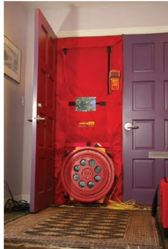
A blower door is used to test the tightness of the house
