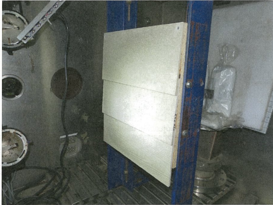
Figure 1. Test specimen made up of three sections of siding fastened to OSB backing plate and wall studs on 16 inch centers (wall studs not visible in photo).
