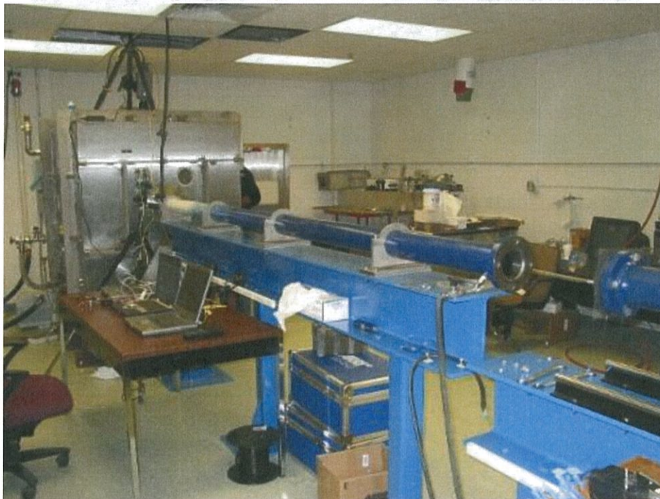
Figure 3. Large vacuum gun (shown with 3 inch diameter gun barrel)
