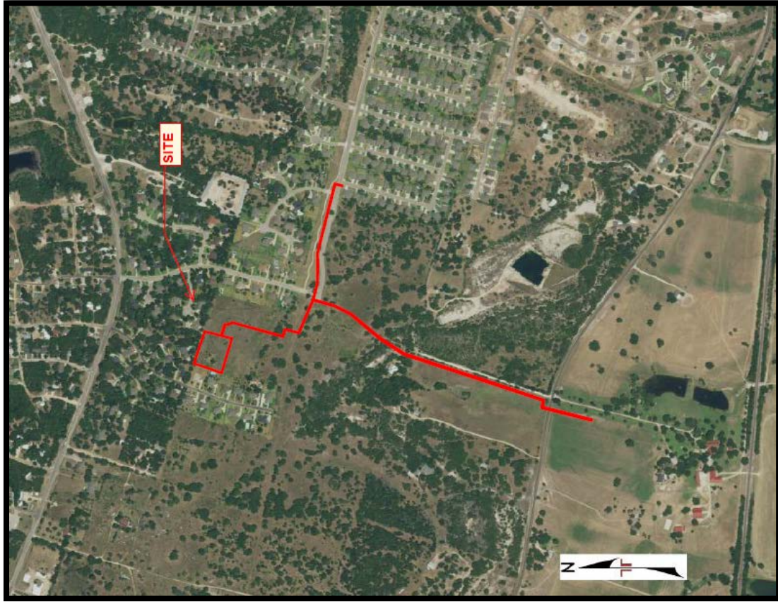
16" North Belton Waterline
