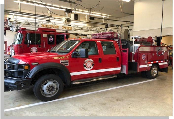
At first glance, the body looks faded and scratched from the rough terrain this vehicle has responded to. At closer examination, the rubber seals on for the compartment doors are dry rotted and are worn to a point of ineffectiveness. There is a moderate to major dent in front of the passenger side rear tire. The safety reflective
