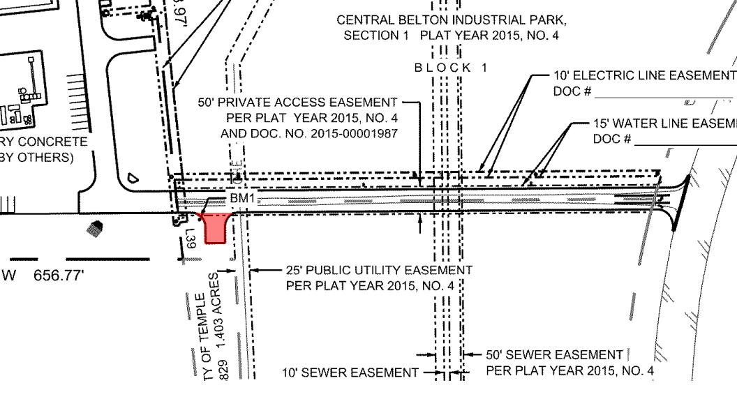
BULLET ITEM #2: CONCRETE DRIVEWAY STUB OVER TO BELTON WASTEWATER TREATMENT PLANT - SHOW RED IS APPROX. 2,100 SQFT OF AN 8" THICK SECTION REINFORCED W/HELIX
