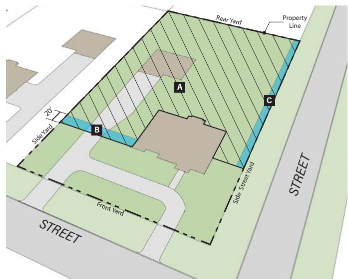
Figure 4.5.2 Rear-yard and Side-Yard Fence Area
