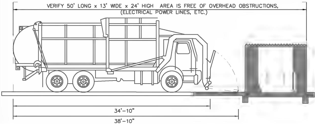
VEHICLE SHOWN IS A STANDARD 40 CY FRONT END LOADING COLLECTION TRUCK. ACTUAL DIMENSIONS WILL DIFFER BASED ON TRUCK MANUFACTURER. COORDINATE DESIGN WITH COLLECTION PROVIDER.
