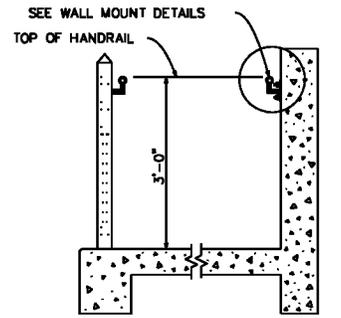
**COMBINATION OF HANDRAIL ON WALL AND RAMP**
