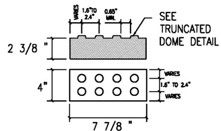
CONCRETE PAVER WITH TRUNCATED DOME SURFACE
