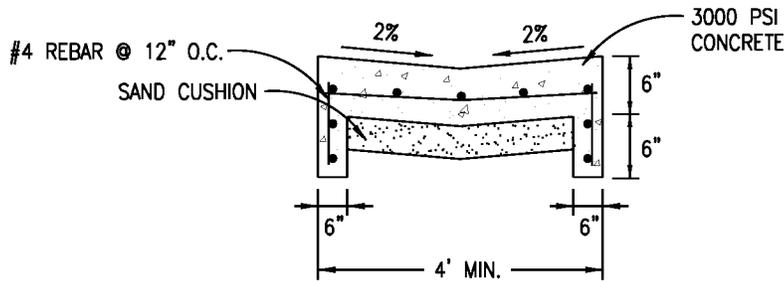
TYPICAL CONCRETE PILOT/TRICKLE CHANNEL
