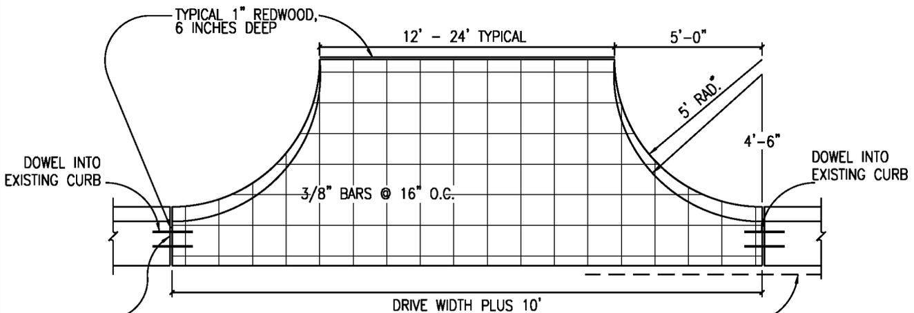
EXISTING CURB TO BE REMOVED TO NEAREST EXPANSION JOINT IF WITHIN 2' OR SAWED TO PROVIDE A CLEAN STRAIGHT LINE.
