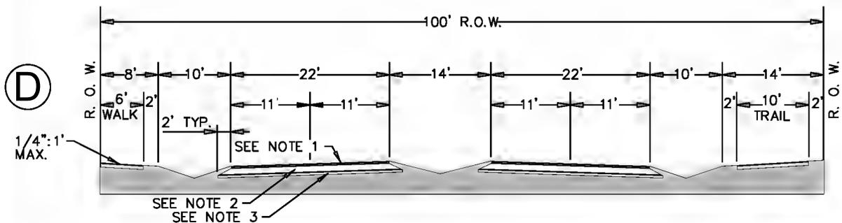
**MINOR ARTERIAL (RURAL CROSS SECTION) - 4 LANE DIVIDED ROADWAY, NO BIKE LANES, 6' SIDEWALK ON ONE SIDE, 10' HIKE AND BIKE TRAIL ON OTHER SIDE**
