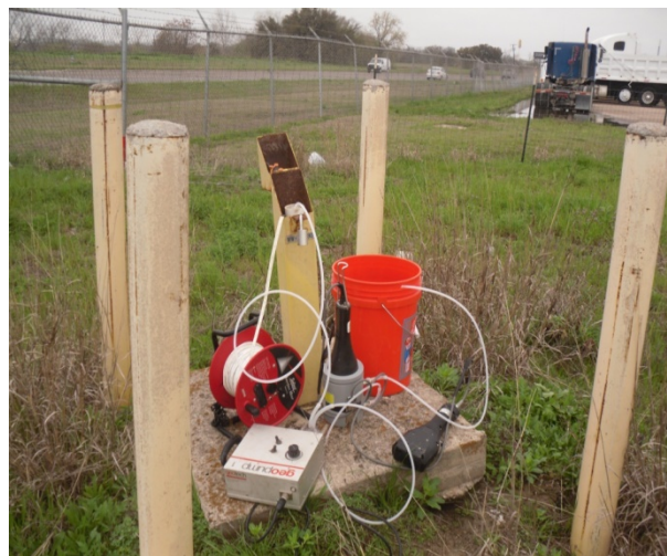
Photo #18 Date: March 19, 2015 Description: Sampling set up on MW-34-90. Facing north.
