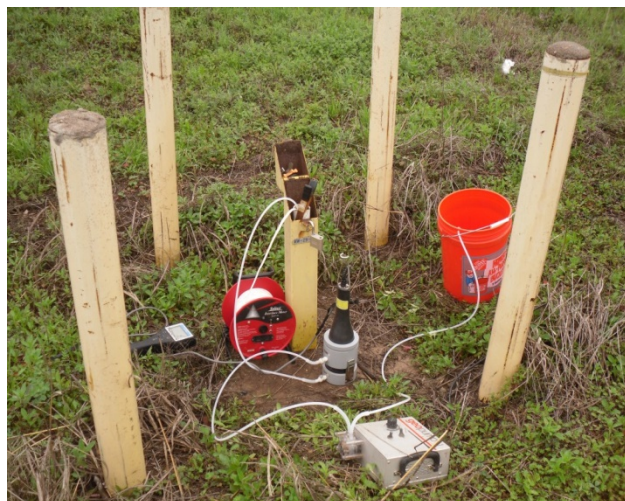
Photo #15 Date: March 19, 2015 Description: Sampling set up on MW-29-90. Facing west.
