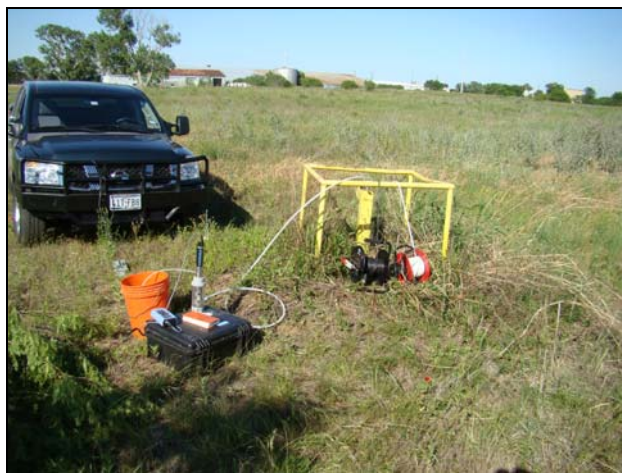
Photo #4 Date: May 4, 2011 Description: Looking Northeast at MW-17 Low-Flow Sampling on the Central Property.
