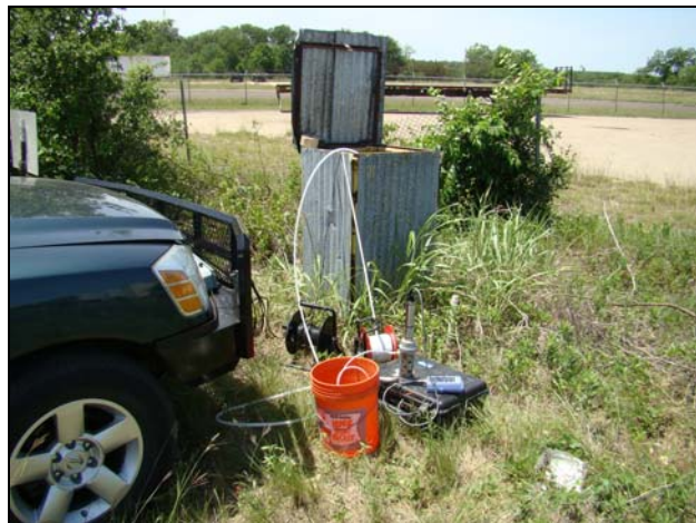
Photo #1 Date: May 4, 2011 Description: Looking Southwest at MW-7 Low-Flow Sampling on the Central Property.
