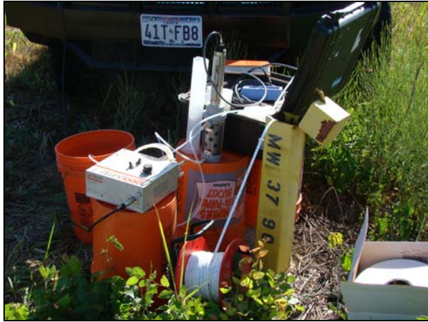
Photo #17 Date: May 3, 2011 Description: Looking East-Northeast at MW-37-90 Low-Flow Sampling on the North Property.
