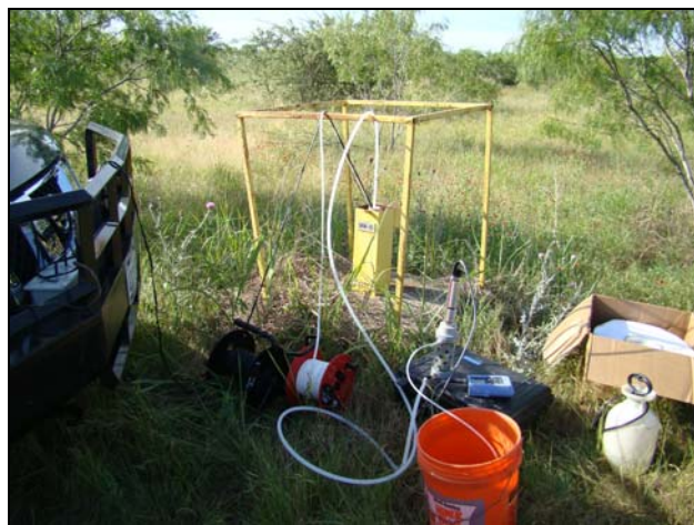
Photo #3 Date: May 4, 2011 Description: Looking West-Northwest at MW-10 Low-Flow Sampling on the Central Property.
