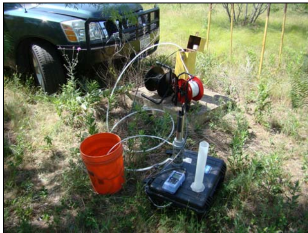
Photo #2 Date: May 4, 2011 Description: Looking Southeast at MW-9 Low-Flow Sampling on the Central Property.
