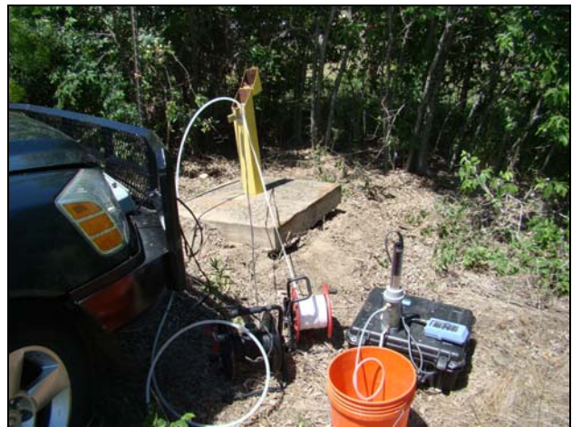
Photo #12 Date: May 4, 2011 Description: Looking Southwest at MW-33-90 Low-Flow Sampling on the Central Property.
