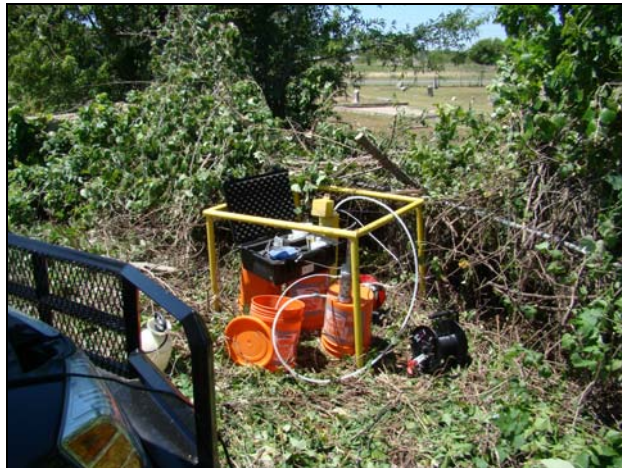
Photo #6 Date: May 3, 2011 Description: Looking Southwest at MW-20 Low-Flow Sampling on the North Property.
