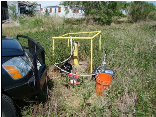
Photo #5 Date: May 4, 2011 Description: Looking Northeast at MW-19 Low-Flow Sampling on the Central Property.
