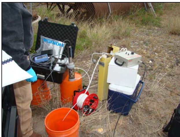
Photo #7 Date: May 2, 2011 Description: Looking Southeast at MW-21 Low-Flow Sampling on the North Property.
