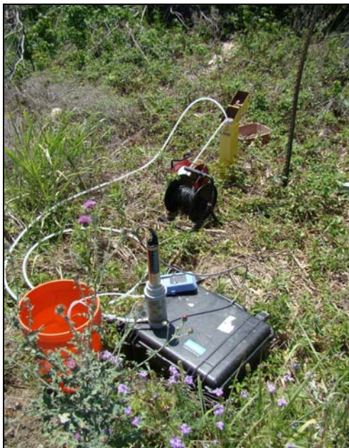
Photo #11 Date: May 4, 2011 Description: Looking Southwest at MW-29-90 Low-Flow Sampling on the Central Property.
