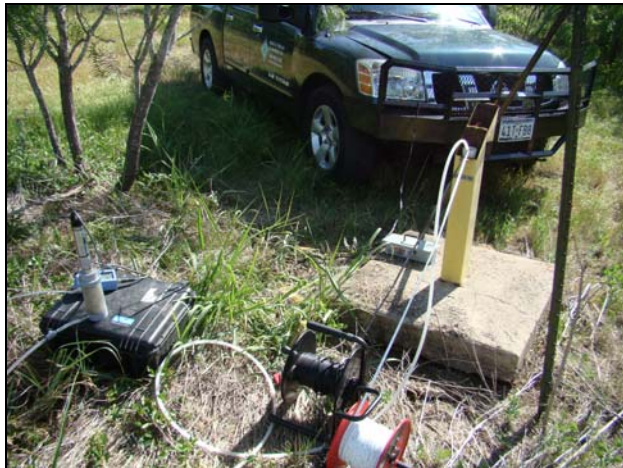
Photo #13 Date: May 4, 2011 Description: Looking North at MW-34-90 Low-Flow Sampling on the Central Property.
