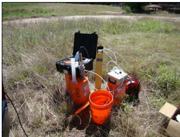
Photo #8 Date: May 3, 2011 Description: Looking East at MW-22 Low-Flow Sampling on the North Property.
