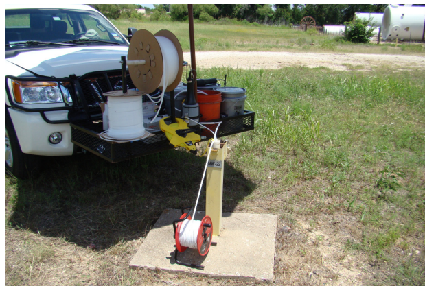
Photo #10 Date: June 11, 2013 Description: Looking southeast at MW-22 Low-Flow Sampling on the North Property.
