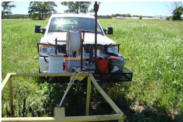
Photo #7 Date: June 10, 2013 Description: Looking west at MW-19 Low-Flow Sampling on the Central Property.
