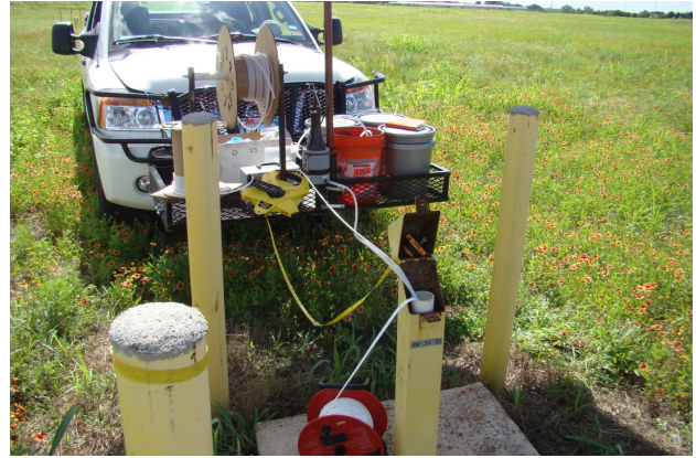
Photo #16 Date: June 11, 2013 Description: Looking south at MW-34-90 low-flow sampling on the Central Property.
