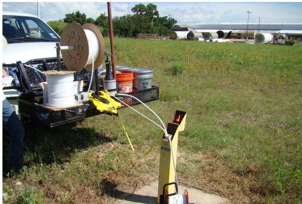
Photo #17 Date: June 11, 2013 Description: Looking south at MW-35-90 Low-Flow Sampling on the North Property.
