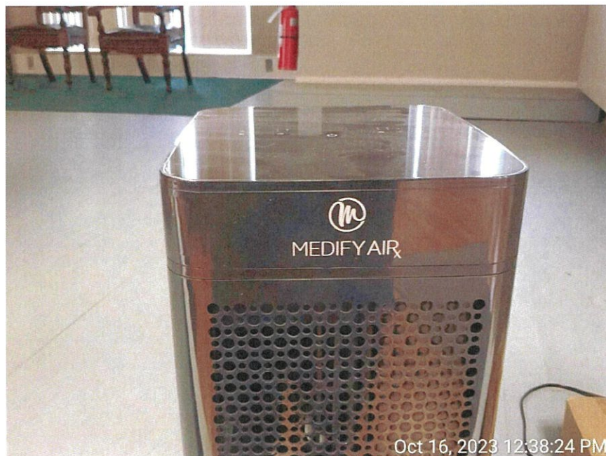
Air purifier on third floor with ionizing setting - Ozone producing.
