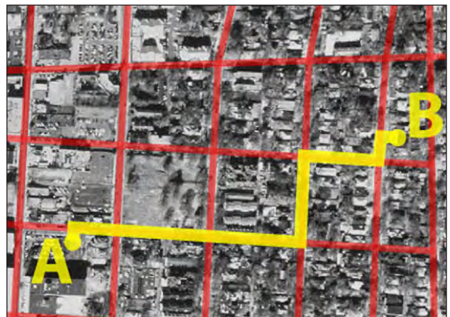
In an interconnected system the distance from A to B is one half mile, with multiple route options
