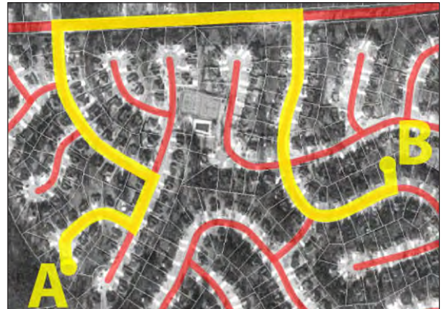
In a dendritic system, the distance from A to B is one mile and achievable along one route
