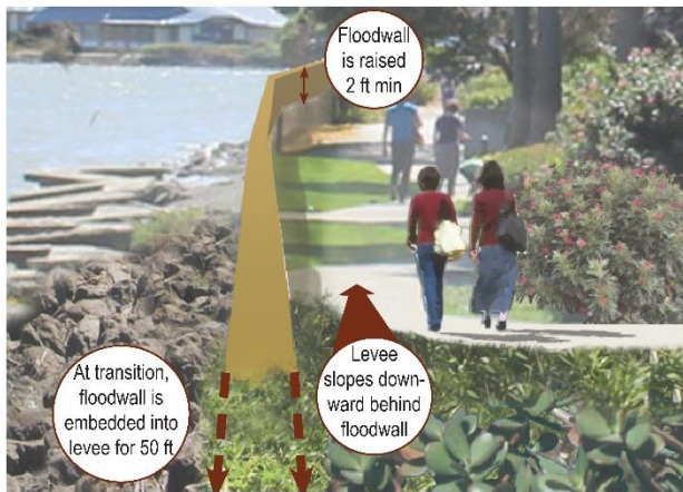
Transition from Levee to Floodwall Detail
