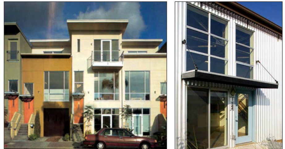
FIGURE 5-11: Design features such as corrugated metal roofs and sidings, simple multi-paned metal rimmed windows, and recycled "green" building materials can maintain the existing varied character of the Myrtle Road Mixed Use Area.
