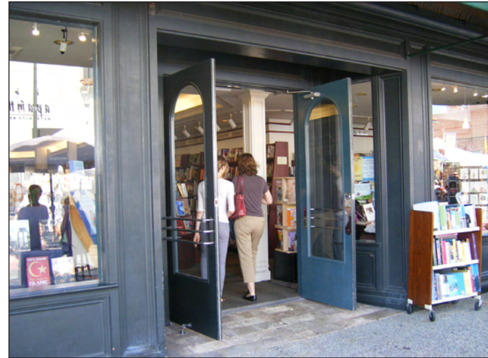
FIGURE 5-3: Commercial entrances should be recessed from the façade, creating a small alcove.
