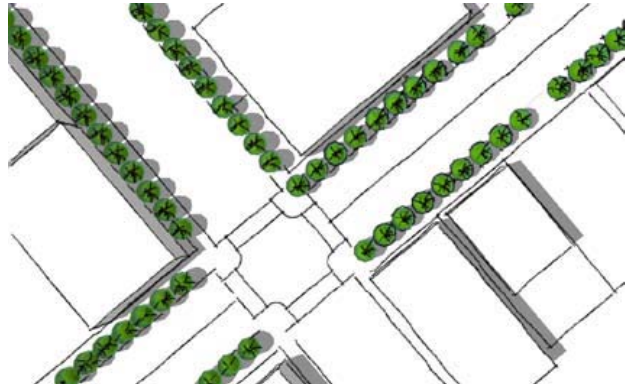
On Howard Avenue wide bulb-outs are recommended at each intersection to provide a more inviting and safer pedestrian experience.
