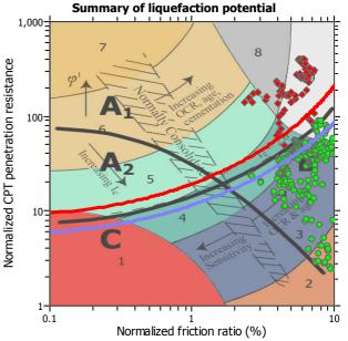
Zone A<sub>1</sub>: Cyclic liquefaction likely depending on size and duration of cyclic loading Zone A2: Cyclic liquefaction and strength loss likely depending on loading and ground
