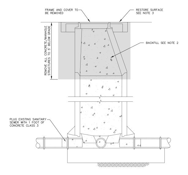
THE EXISTING MANHOLE TO BE ABANDONED IN PLACE SHALL BE AS SHOWN ON PLANS AND IN ACCORDANCE WITH THE FOLLOWING REQUIREMENTS AND STANDARD SPECIFICATIONS:
