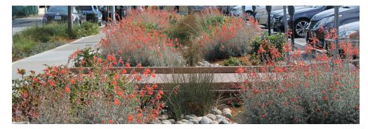
**Bioretention areas** (also called rain gardens) are shallow, recessed, and vegetated basins that collect and absorb runoff from surfaces such as rooftops, sidewalks, and streets. These landscapes contain soil of a specified biotreatment soil mix (BSM) that is designed to slow, retain, and filter stormwater runoff. When stormwater flows into a bioretention area, this prevents pollutants (such as vehicle fluids and trash) from flowing into a storm drain and into the San Francisco Bay.
