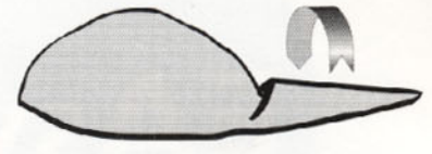
sandbag, open end folded over - side view
