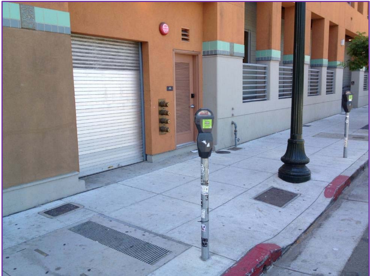
Figure 12. Well-designed trash room access with curb cut and red zone.
