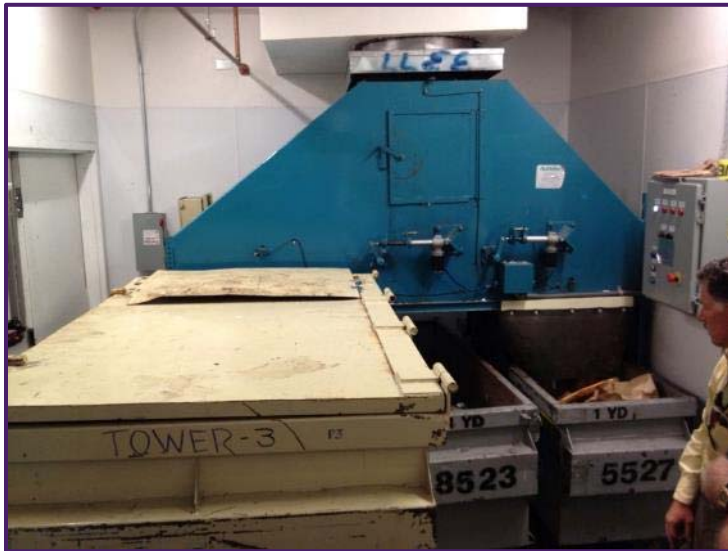
Figure 19. Tri-Sorter with compactor for garbage.
