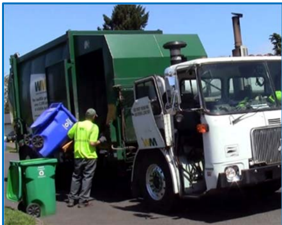
Figure 25. Side-loading vehicle tipping carts into hopper with good wind protection
