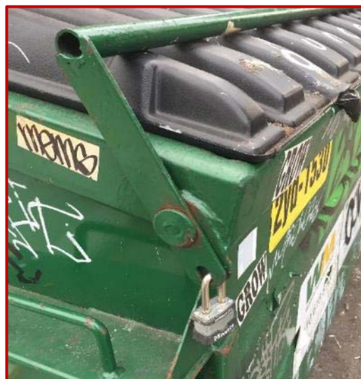
Figure 30. Locking lid on Front End Load (FEL) container.
