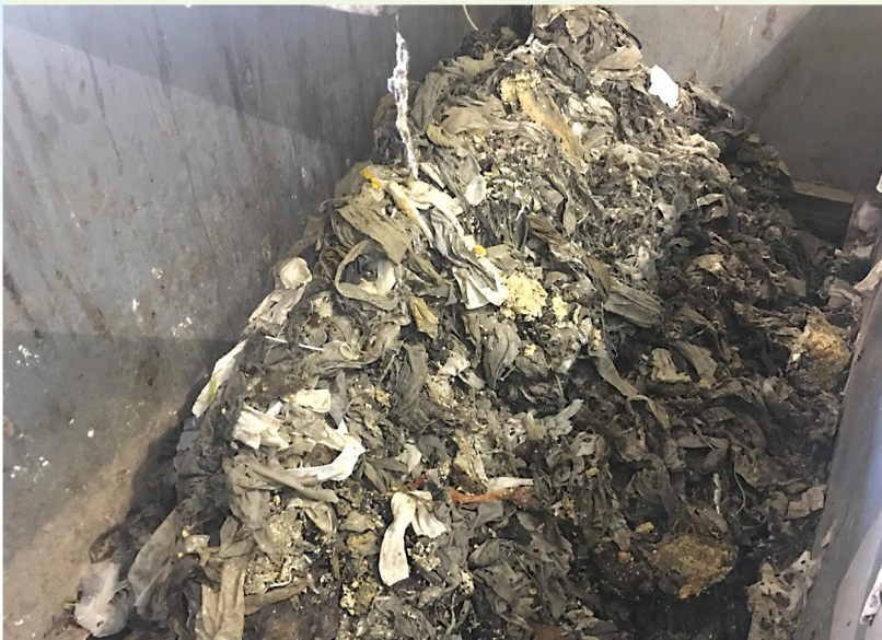
Used “flushable” wipes and other items removed from a sewer in Clinton Township by the Macomb County Public Works Office.
