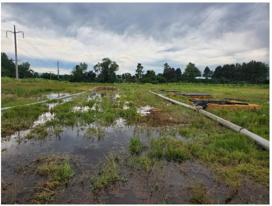
*Photo 5 – Groundwater Discharge during Constant-Rate Testing.*
