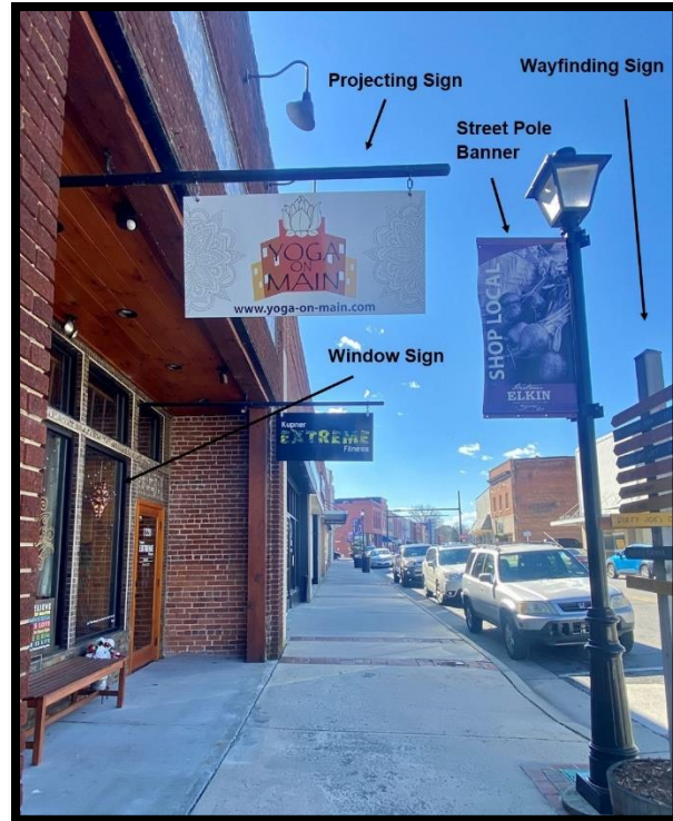
Figure 7.1 Examples of Signs, Including Projecting Signs, Street Pole Banners, Wayfinding Signs, and Window Signs.
