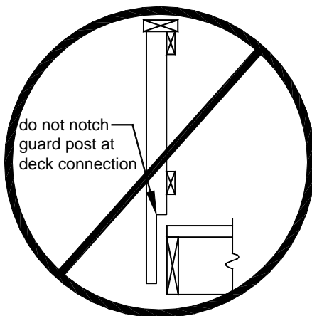
FIGURE 29: NOTCHING AT GUARD POSTS
