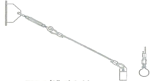
TRB 1/2"-4' Cable Support TRB 3/4"-4' Cable Support
