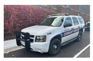
Community Service Officer vehicle and was repurposed after serving as a patrol vehicle. Patrol vehicles accrue significant idle time which creates additional stress on engine components. As such, the potential for failure in the engine and drivetrain increases as patrol vehicles approach these thresholds, as do the repair costs over and above preventive maintenance. Due to the repurposing of the vehicle from patrol fleet, the vehicle is 8 years old and has extensive rust and body deterioration.
