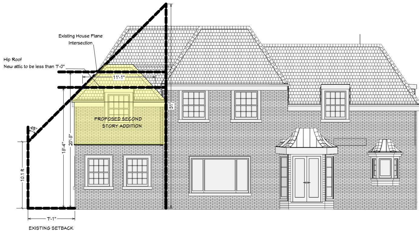
SETBACK PLANE AT SOUTH ELEVATION
