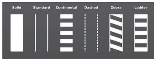
Examples of a variety of crosswalk marking designs. Source: Federal Highway Administration
