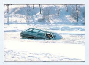
An insurance company staged this breakthrough for a water safety film. The car sank within 45 seconds, turned over, and settled on its top.
