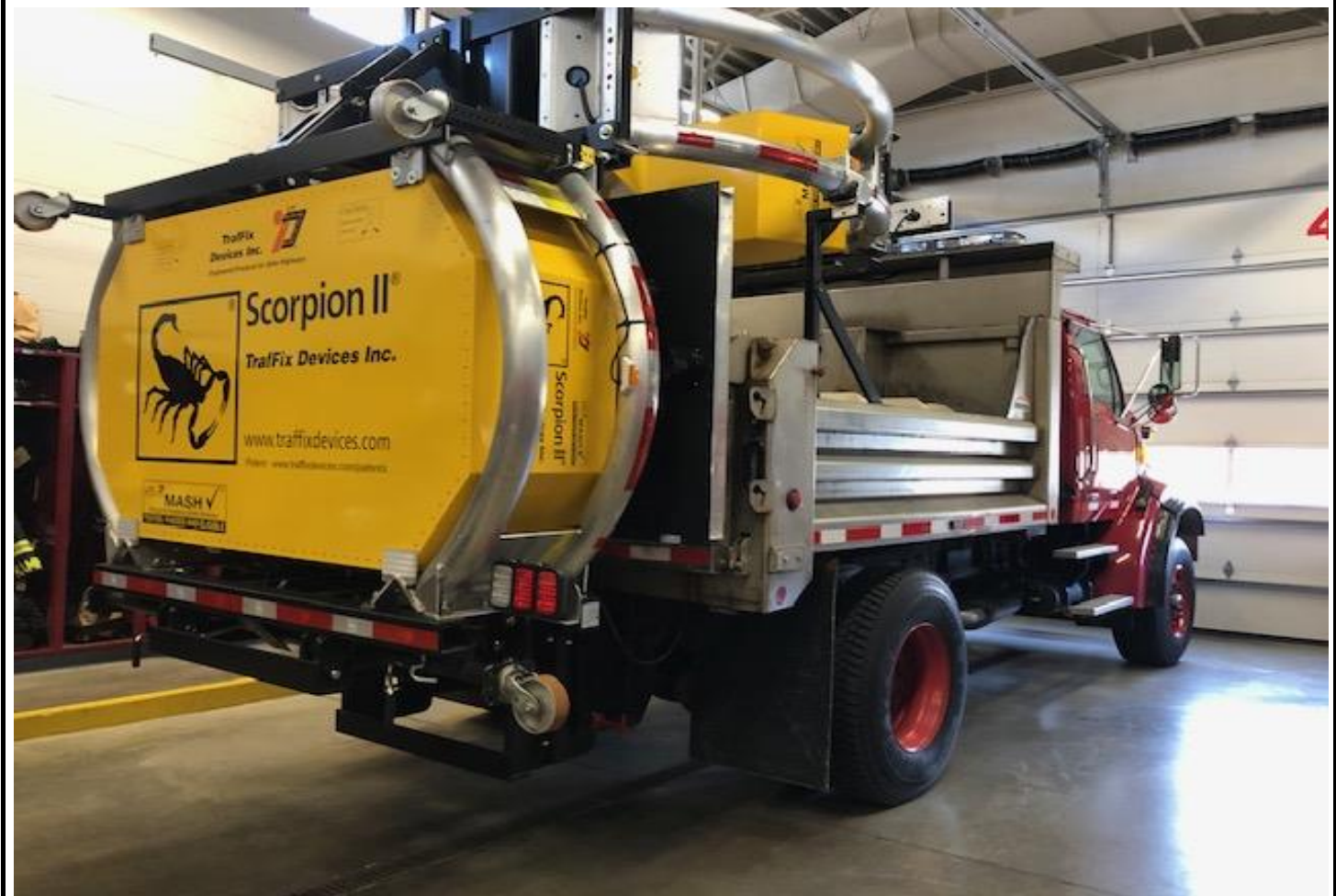
"Dumpy" traffic attenuator ready to respond (above) and deployed on an accident on East Beltline near 28th on March 11, 2024.
