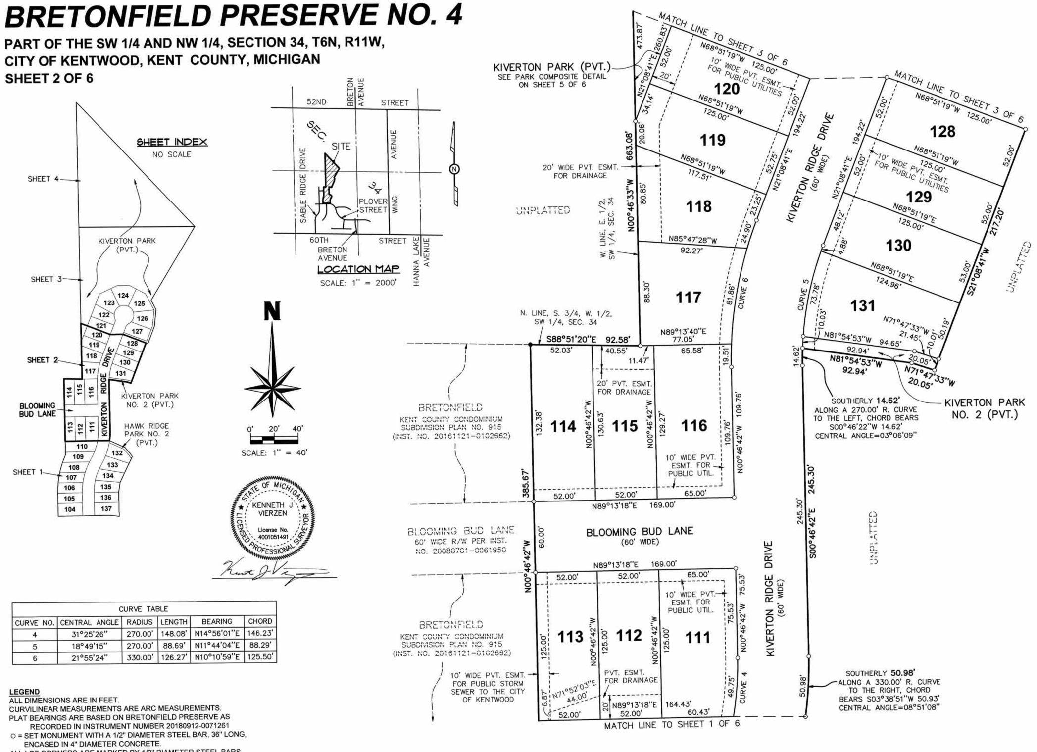
ALL LOT CORNERS ARE MARKED BY 1/2" DIAMETER STEEL BARS, 18" IN LENGTH WITH SURVEY CAP MARKED EXXEL 50433. R = RADIAL. LINES NOT MARKED ARE NON-RADIAL.
