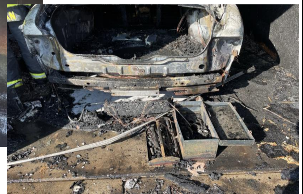
Changing fuel pump in attached garage. Fire damage in garage; smoke in interior.
