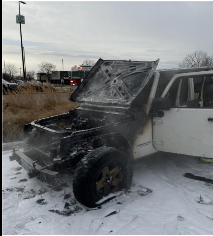
Fire in engine compartment of Jeep Wrangler extended into passenger compartment. Minor heat damage to VW parked nearby.
