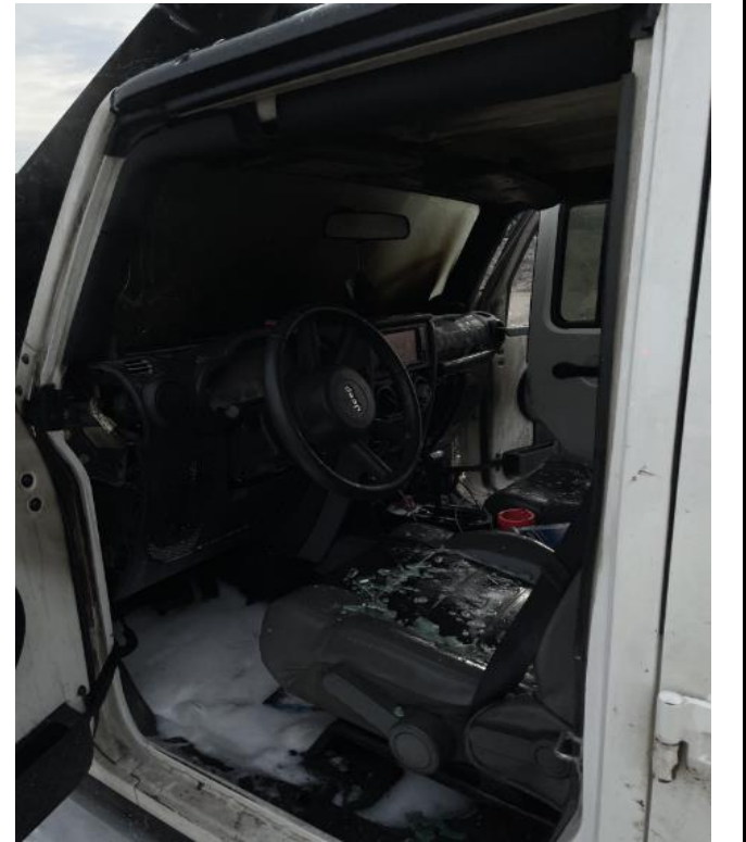
Fire in engine compartment of Jeep Wrangler extended into passenger compartment. Minor heat damage to VW parked nearby.
