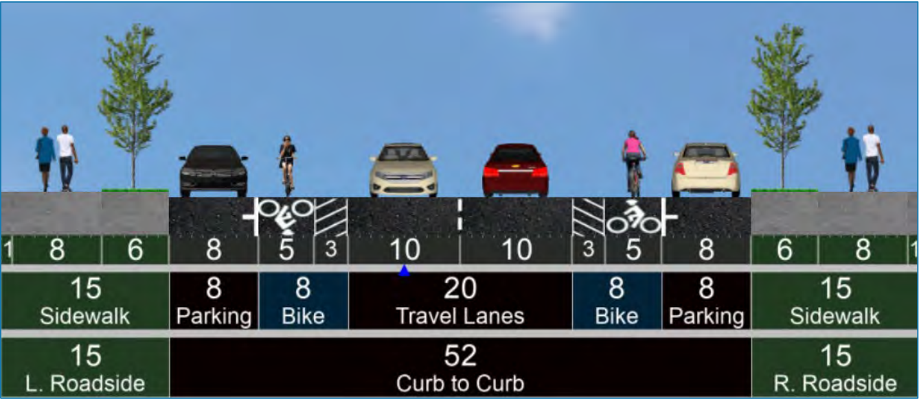
FIGURE 32: TYPICAL CITY COLLECTOR, NEIGHBORHOOD ROUTE, AND LOCAL STREET CROSS-SECTION WITH MULTIMODAL AREA (RESIDENTIAL) AND NEIGHBORHOOD BICYCLE ROUTE DESIGNATION
