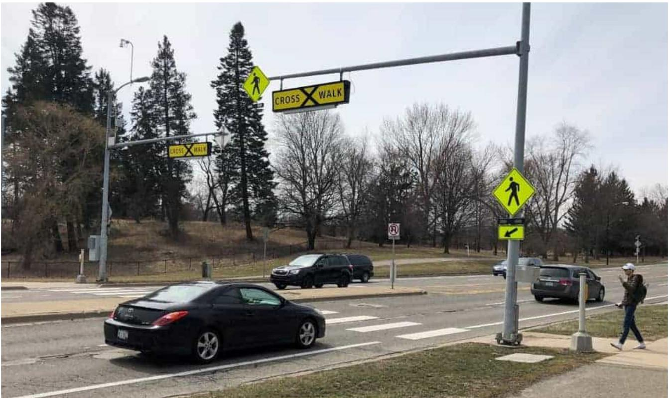
*Rectangular Rapid Flashing Beacon and pedestrian crosswalks support the safety of pedestrians at crossings*
