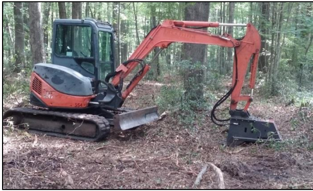
Figure 28. Hitachi mulcher used to breakdown piece size of cut vegetation. Credit: ANF.
