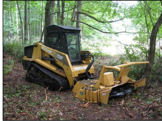
Figure 29. Skid Steer used to remove vegetation for mulching. Credit: ANF.
