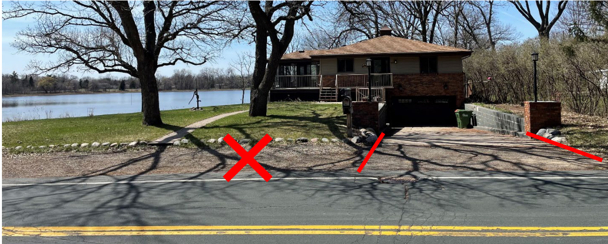
7830 Spring Lake Road (photo April 18, 2023). Non-conformity: ROW is used for parallel parking, whereas no parking is allowed. Homeowner has requested a Variance for a 2nd curb cut to allow a horseshoe driveway with a 0' front yard setback (Minimum of 5' required). This Variance would need to be approved by the Planning Commission because it is new construction. The existing gravel parking area will be displaced by the trail. Proposed driveway would be located in between the boulder retaining wall and the two trees. Staff is recommending a parking pad, vs a horseshoe driveway.
