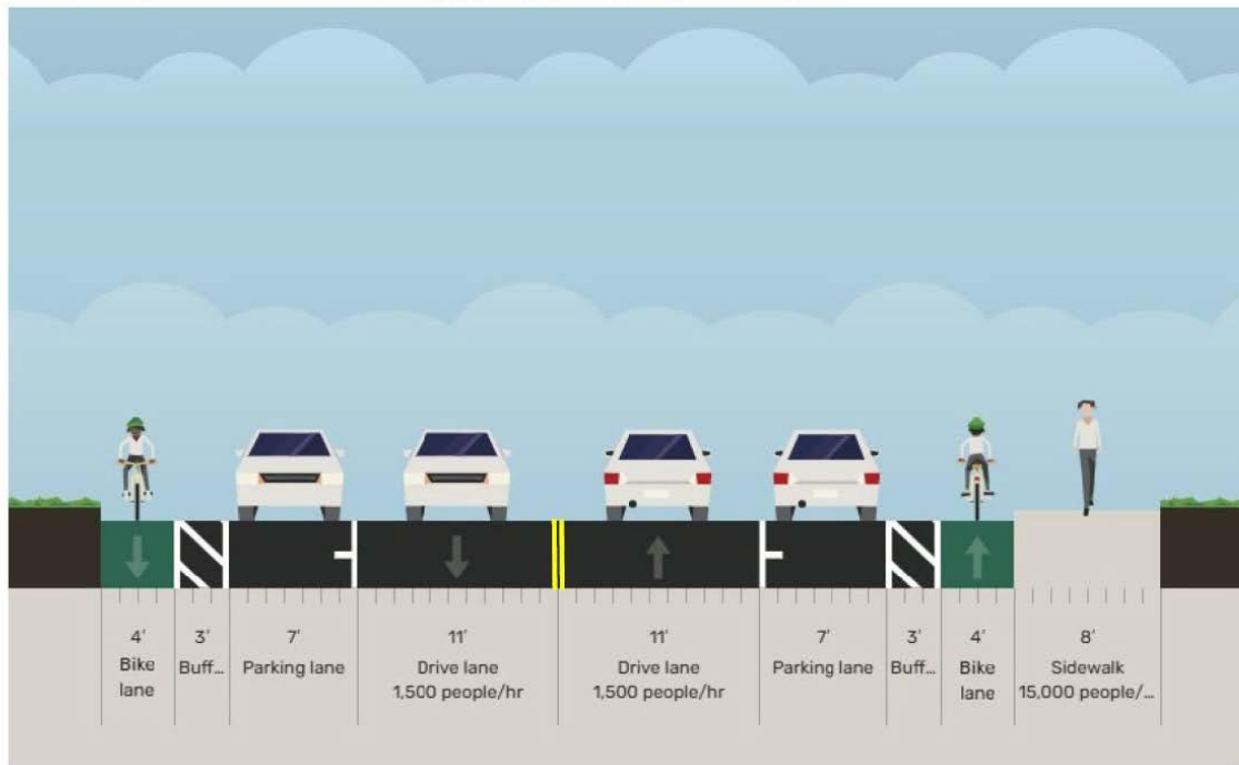
Parking-protected bicycle lane with buffer (north of 115 Kisco Avenue) – looking north
