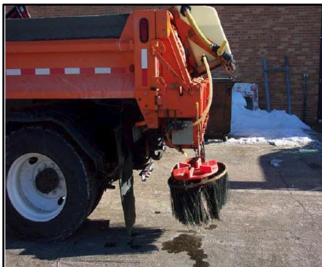
Figure 15: Salt skirt retrofitted on a municipal truck to target salt application at the center line. Source: Minnesota DOT.
