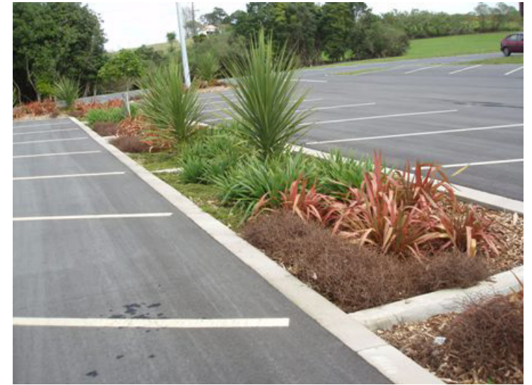
Use of native plants within landscape areas of parking lots can aid in removal of contaminants and sediments from stormwater prior to drainage into the watershed.
