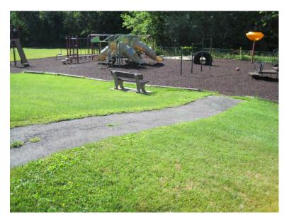
The ramp leads to a paved path shown in the above photo. The path is of a steep grade and is rough in certain areas. Appropriate regarding of the path is needed to meet accessibility requirements.
