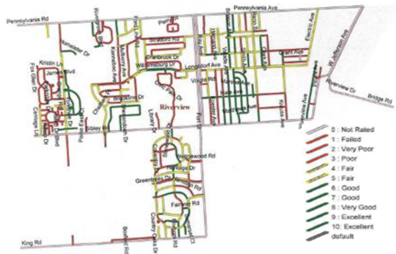
Figure 8: Road Surface Conditions
